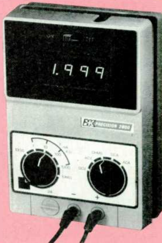
Digital multimeters are most often advertised as having 3½-digits or 4½-digits, which refers to the fact that the most-significant-digit (far left) can display a 1 or 0 only.
