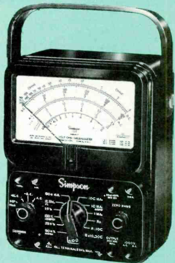
The Simpson 260-type VOM is probably the most famous of all, having served as the archtypical design for many others, both more and less expensive. It is the "reference standard" VOM.
