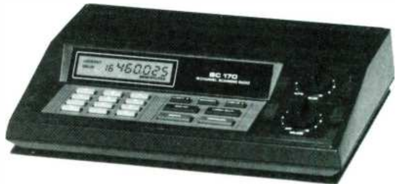
The Uniden Bearcat BC-170 is capable of receiving 11 frequency bands, and its LCD display shows the frequency being programmed or monitored, as well as operation modes—all at a suggested retail price of $229.95.
